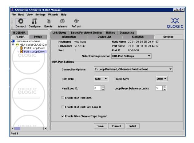
Use this procedure to verify that Fiber channel tape support is enabled.
