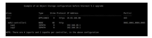
Figure 2: Example of a DDM Object Storage device configuration before a StorNext 5 release 5.1 upgrade
