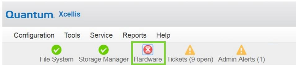
When clicked, this hardware failure displays multiple fan failures on the **System Board** tab of the **Reports > Hardware Status** in the StorNext GUI:
