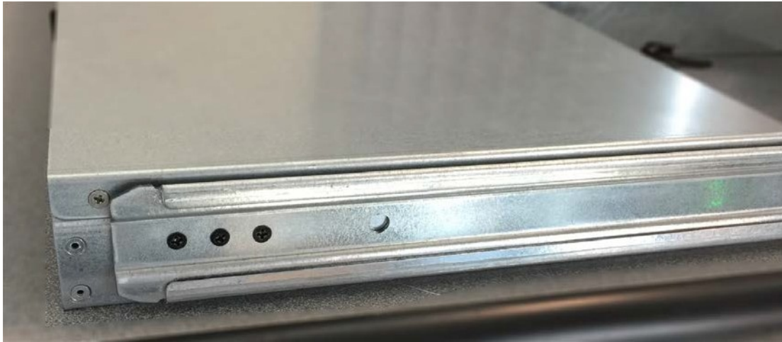
Figure 3-88. Screws on Management Interconnect tray rail
