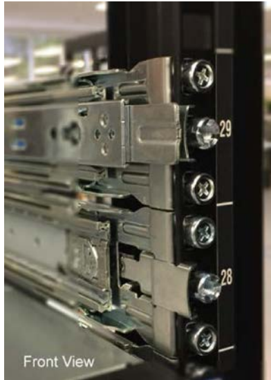
Figure 8-4. Rail attaching to front vertical rail
