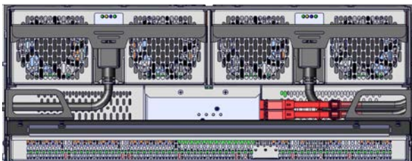
Figure 11-42. Removing the HD Mini-SAS cables
