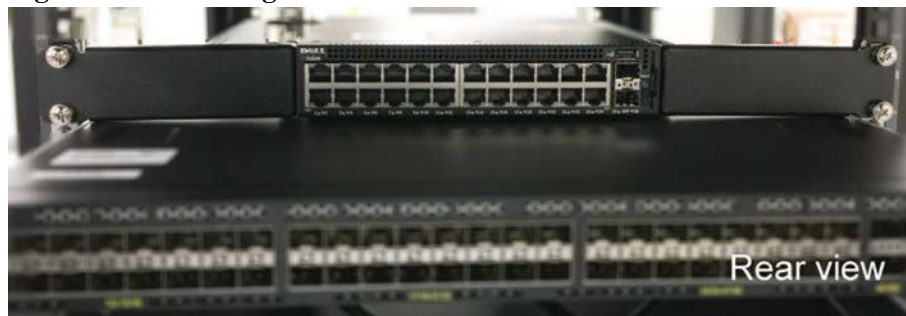
Figure 3-21. Management Interconnect rack ears
