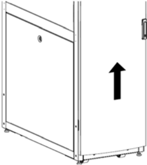
Figure 3-101. Uninstalling the rack door
