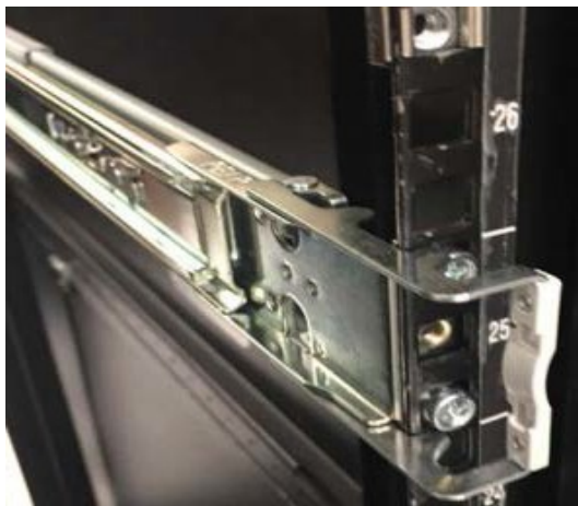
Figure 8-3. Rail attaching to rear vertical rail
