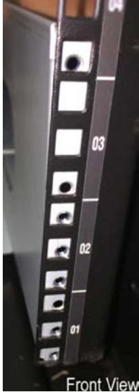
Figure 3-96. Front Rail Flush Behind Front Vertical Rail
