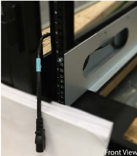
Figure 3-100. Power Cable Routing to Front of Cabinet
