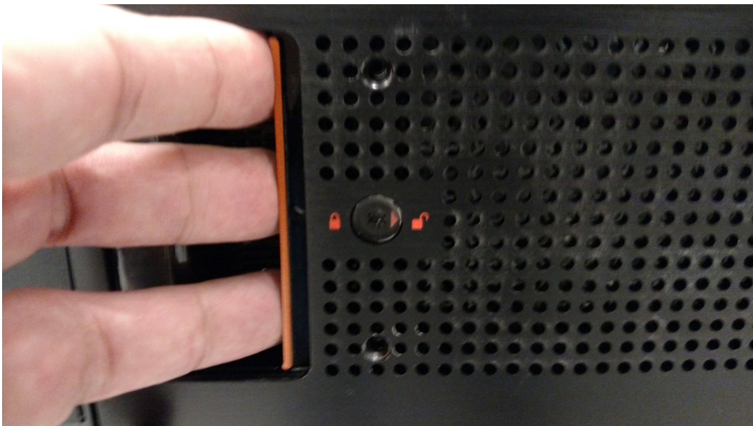
Figure 158 5U84 Chassis Bezel Drawer Latches (2 Each)
