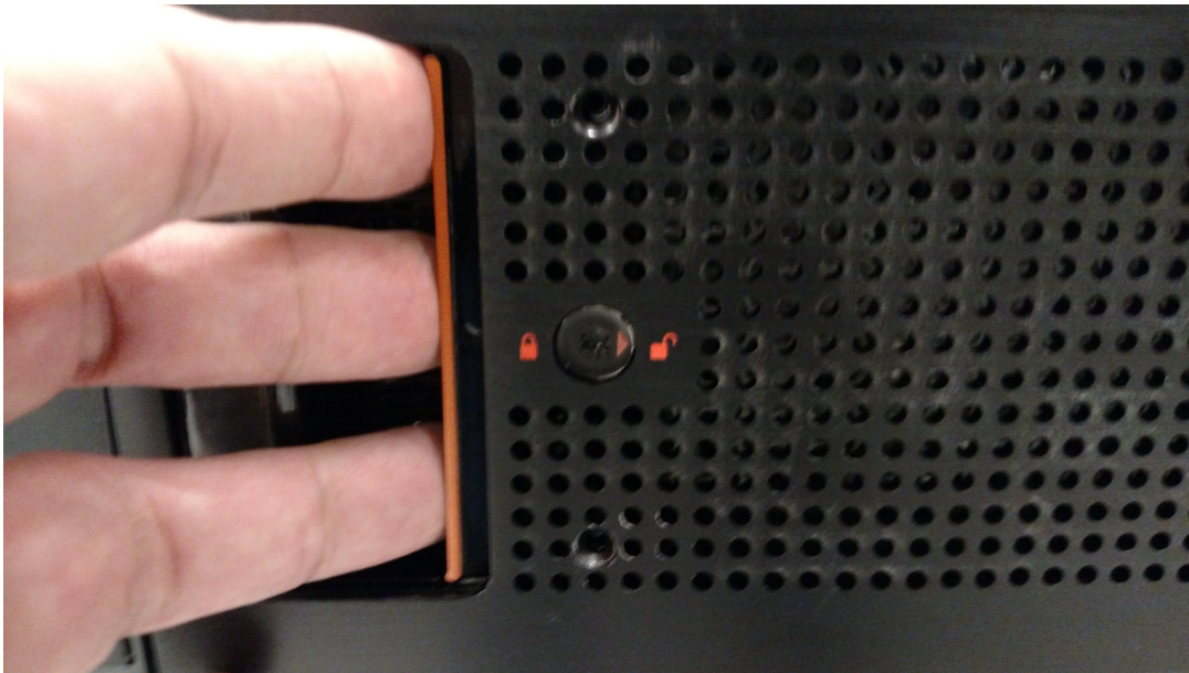
Figure 162 5U84 Chassis Bezel Drawer Latches (2 Each)
