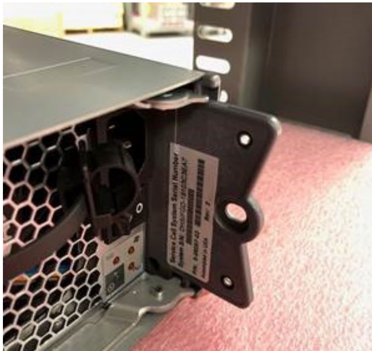
Figure 7 Serial Number Label on Right-rear Ear of Chassis
