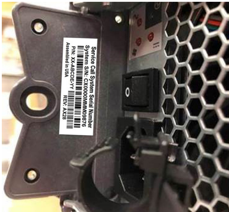
Figure 6 Serial Number Label on Left-rear Ear of Chassis
