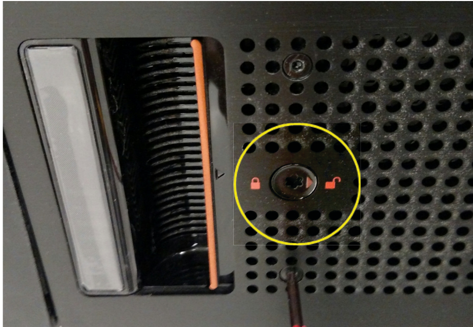
Figure 161 5U84 Drawer Unlock Anti-tamper Locks
