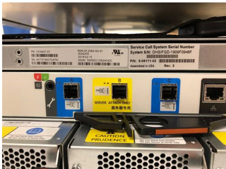
Figure 14 5U84 System Serial Number Label Location
