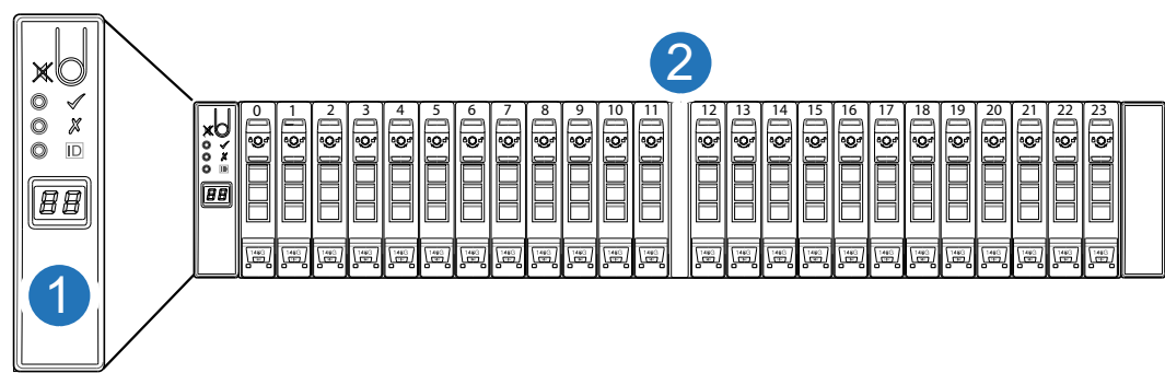
Figure 36 2U24 Chassis Ops Panel
