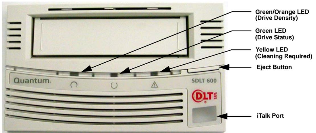
On the SDLT 600 tape drive, the leftmost LED is dual color (green/orange). This LED is the Density Indicator. When you insert a Super DLTtape II data cartridge, this LED illuminates green. When the tape drive detects a backward read compatible (BRC) data cartridge, this LED illuminates orange. (For BRC details, see [Backward Read Compatibility \(BRC\) Transfer Rates](#) on page 34.)
