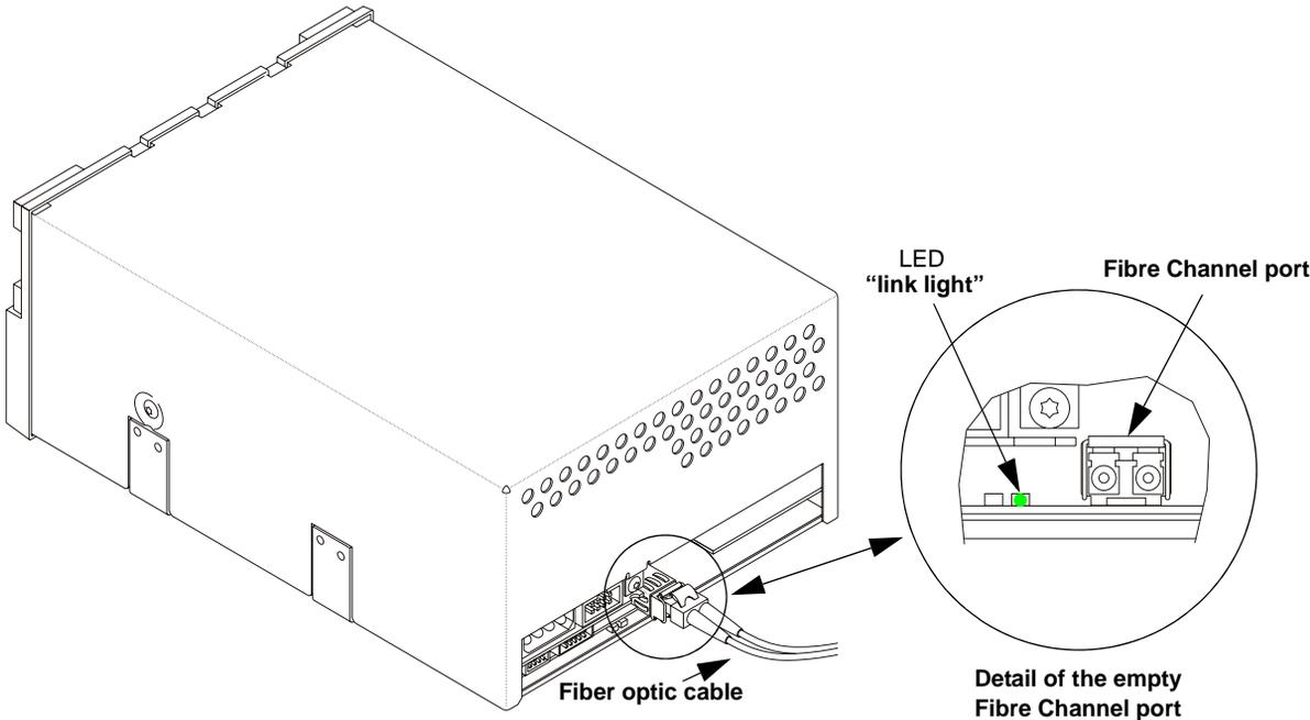
**Note:** You can connect a Fibre Channel connector while the tape drive is still powered on; this capability is known as "hot-swappable" or hot-pluggable." When connecting to the Fibre Channel port, make sure to use a 50µM Fiber core fiber optic cable with an LC, Duplex connector.
