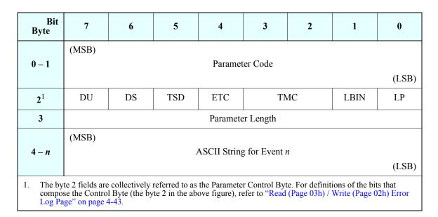
Figure 4-22. Log Parameters Format for Last *n* Error Events LOG SENSE Page
