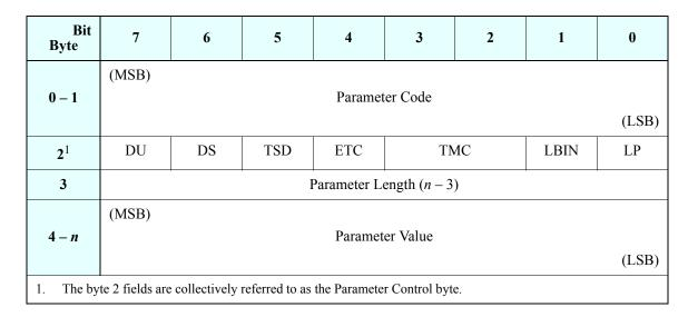
Figure 4-16. LOG SELECT Log Page — Parameters Format
