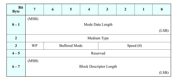
Figure 4-61. MODE SENSE (10) Data Header — Data Format
