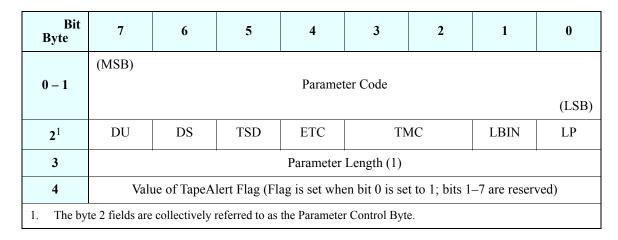
Figure 4-28. TapeAlert LOG SENSE Page — Parameters Format
