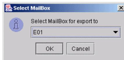
After a cartridge has been moved to the mailbox slot through the **Export** command and become *ejected*, it cannot be manipulated again until **Inventory** has been completed. After an **inventory** is completed, the cartridges are recognized as *stored*.
