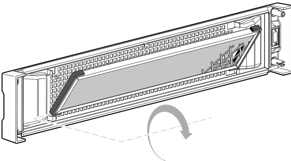
4. Carefully extract the air filter from the bezel.
