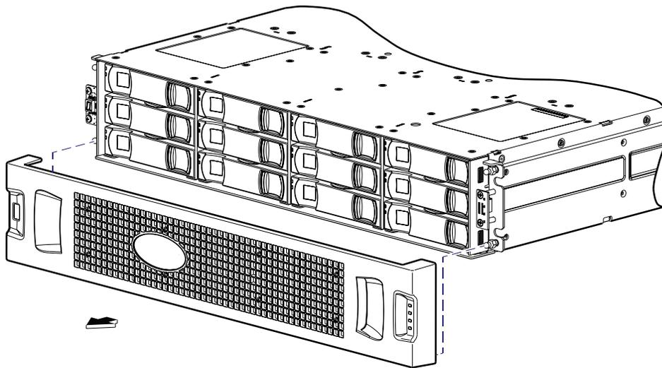
2. While holding the bezel in one hand, gently slip your thumb or index finger between the top of the filter frame and its foam insert on the back side of the bezel.
