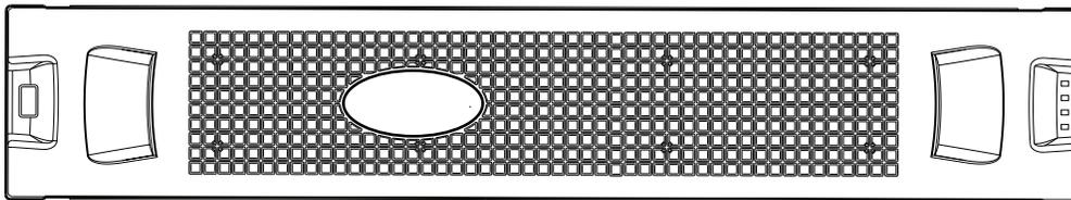
**Figure 2:** Optional air filter sub-assembly - front view
