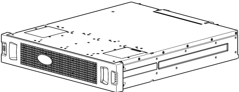
5. Gently push-fit the two ear cover areas of the bezel onto the ball studs to secure the bezel in place.
