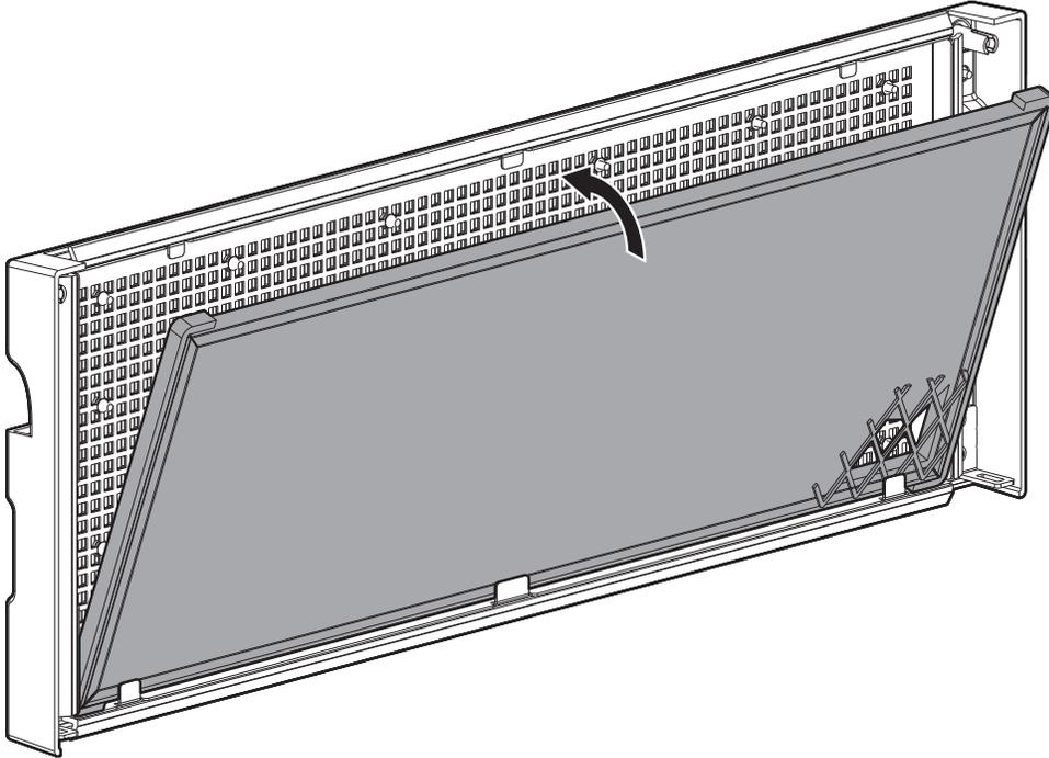
Once properly seated — and revolved into position — the installed air filter should appear as shown in the figure below; albeit with visible foam-retaining mesh in front of the shaded foam insert (the mesh is only partially shown in the illustrations provided in this document).
