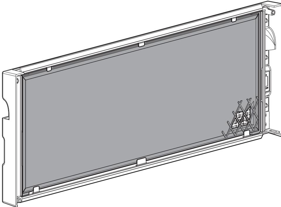
**i Note:** Once the air filter is successfully installed within the bezel, you can reattach the bezel to the front face of the chassis.
