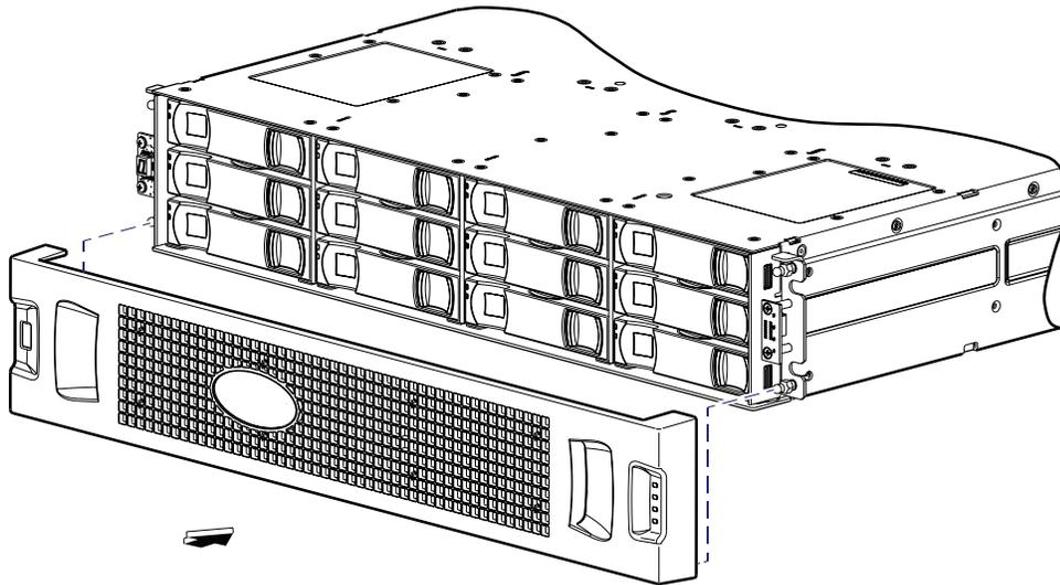
4. Face the front of the chassis, and while supporting the base of the bezel, gently slip the integrated ear covers onto the push-fit ball studs, taking care to guide the LED indicators through bezel openings.
