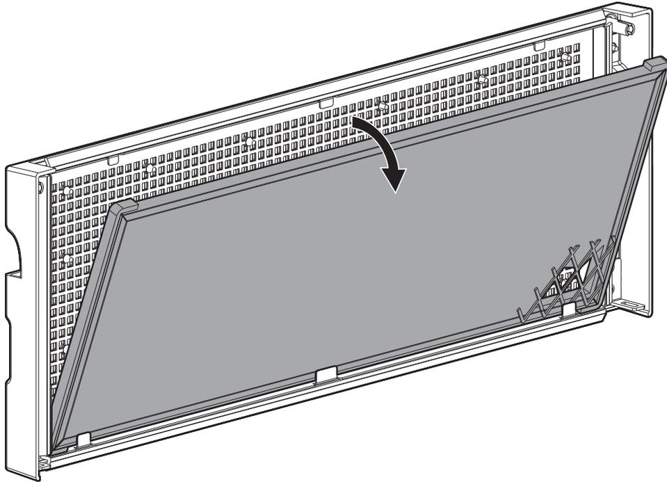
4. Carefully extract the air filter from the bezel.
