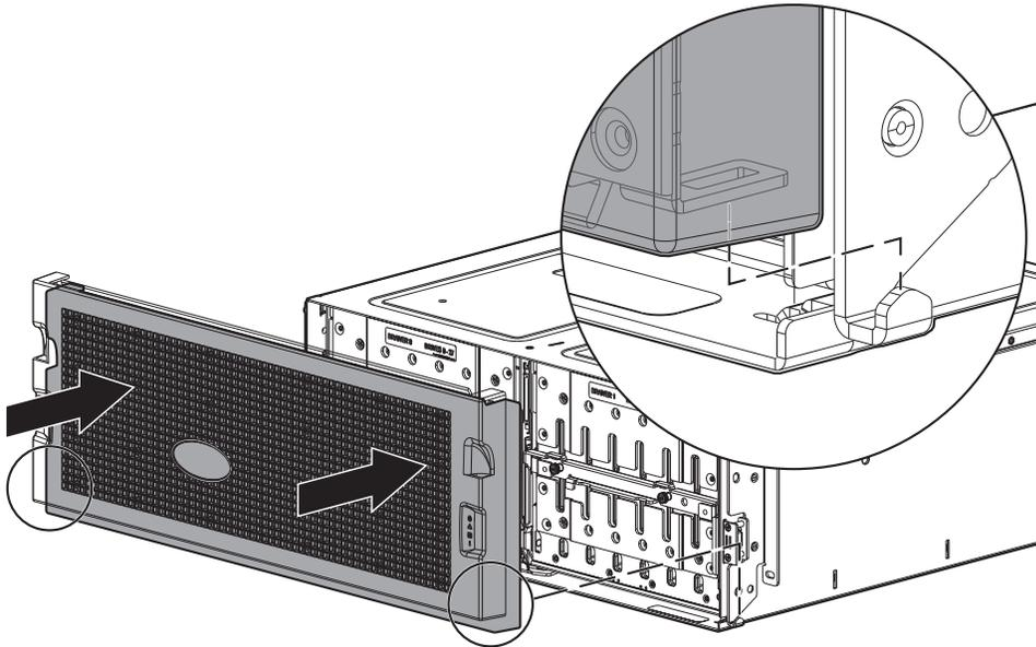
4. Face the front of the chassis, and while supporting the base of the bezel, gently slip the integrated ear covers onto the push-fit ball studs, taking care to guide the LED indicators through bezel openings.
