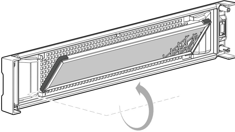
Once properly seated — and revolved into position — the installed air filter should appear as shown in the figure below; albeit with visible foam-retaining mesh in front of the shaded foam insert (the mesh is only partially shown in the illustrations provided in this document).
