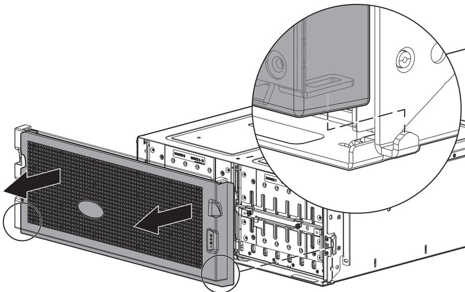
2. While holding the bezel in one hand, gently slip your thumb or index finger between the top of the filter frame and its foam insert on the back side of the bezel.
