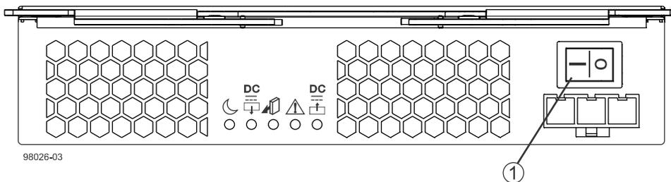
1. Power Switch for the DC Power-Fan Canister
