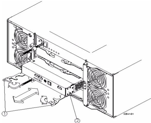
While removing the ESM canister, you might notice an increase in fan speed. The fan speed returns to normal after you have replaced the ESM canister.
