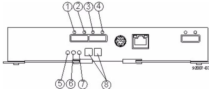
1. ESM Link Fault LED (Port 1A Bypass) (Green)
