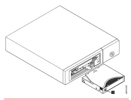
**Caution:** Do not attempt to load a cartridge when the drive is in Maintenance Mode until the drive requests it.
