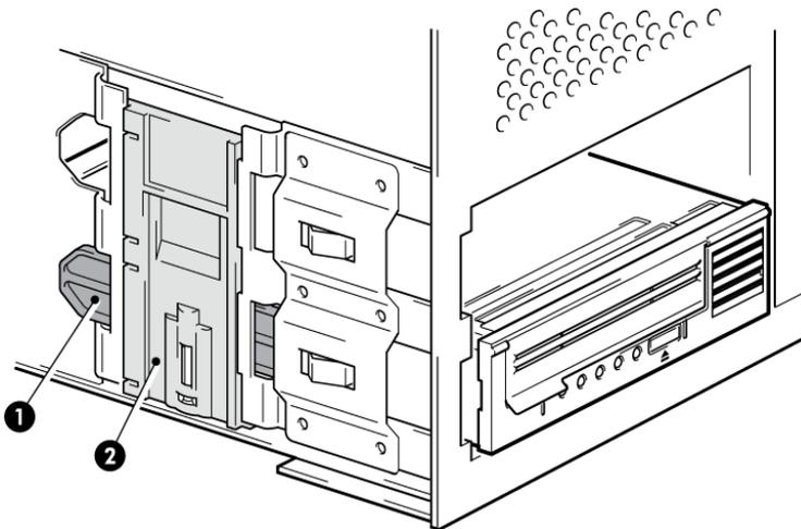
Figure 4 Installing tape drive
