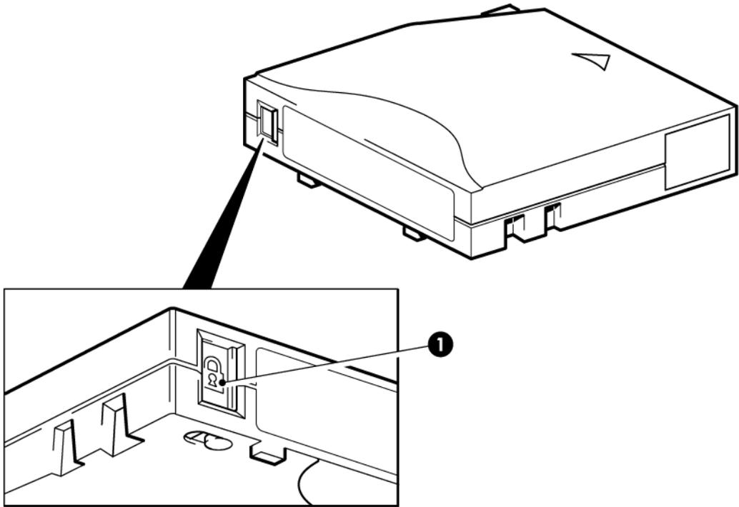
1. Write-protect tab (padlock indicates cartridge is protected)
