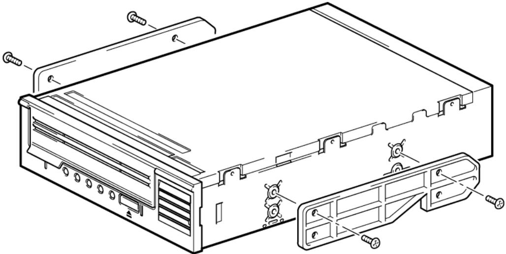
Figure 2 Attaching mounting rails to a half-height tape drive
