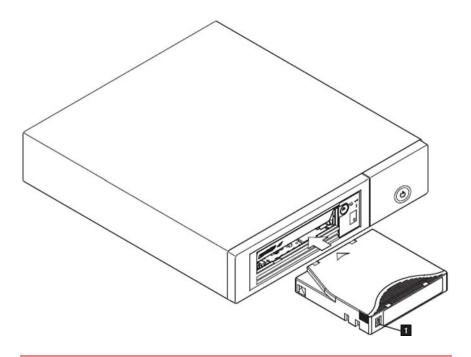
**Caution:** Do not attempt to load a cartridge when the drive is in Maintenance Mode until the drive requests it.
