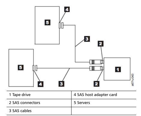
4 Ensure the host adapter and the server are configured correctly for a SAS bus operation. Refer to the host adapter and server documentation for instructions.
