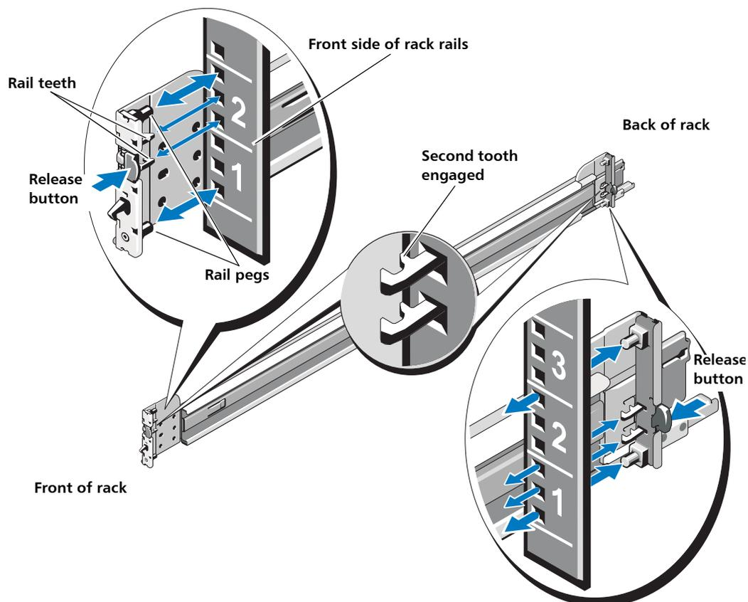
Figure 4 Installing the Rack Mounting Rails (Round Holes)
