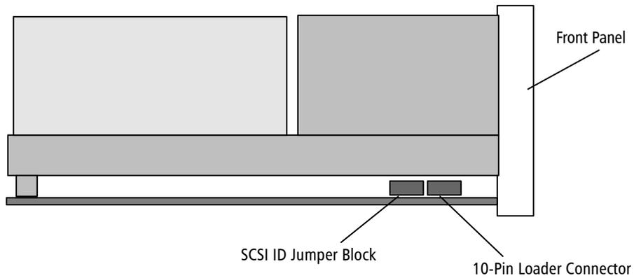
Figure 2-5 Loader Connector Block Location (Rackmount Version Shown)
