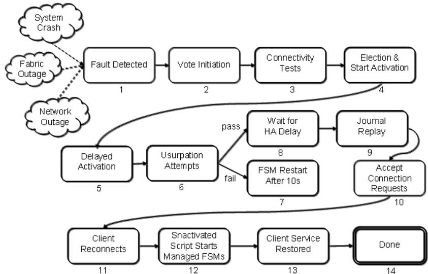
Not shown in this diagram are the state transitions of the peer MDC when it incurs an HA Reset. The HA Reset is not directly tied to the failover of control to a standby FSM, but rather the detection of a loss of services triggers failovers. The HA Reset may come before or after the loss of services, or not at all. It is only important to know
