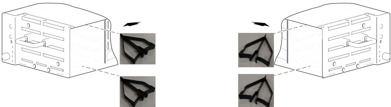
1. Squeeze the latch release flanges together—so that the locking-nib will clear the sheet metal bay wall—and insert the AMS into the target drive bay.
