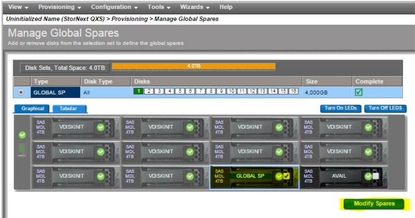
3. As soon as the drive is added to the Global Hot Spare group, the LUN rebuild process initiates automatically.
