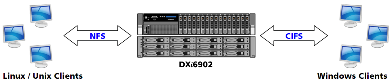
Figure 12: NAS Backup using CIFS/SMB and NFS
