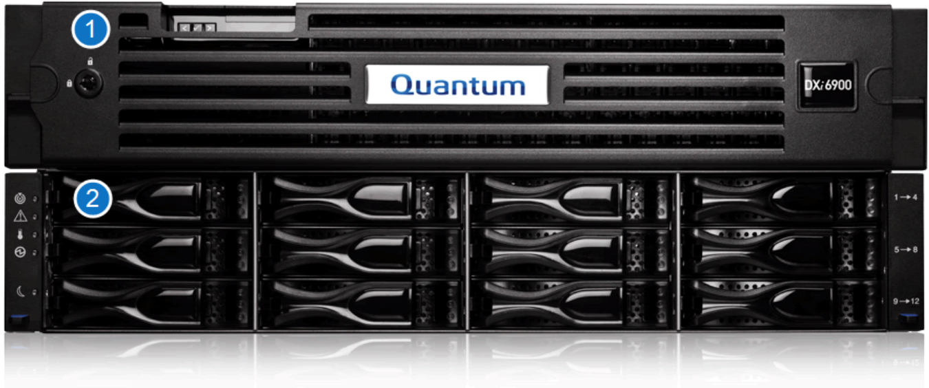
1. DXi6900 Node 2. Array Module (RBOD)/Expansion Module (EBOD)
