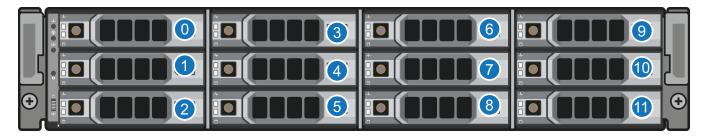
Figure 7: DXi4700 G2 Expansion Module Drive Slot Numbering
