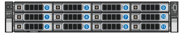
Figure 5: DXi4700 Node Drive Slot Numbering
