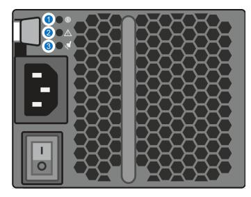
1 - DC Power 2 - Power Supply Fault 3 - AC Power
