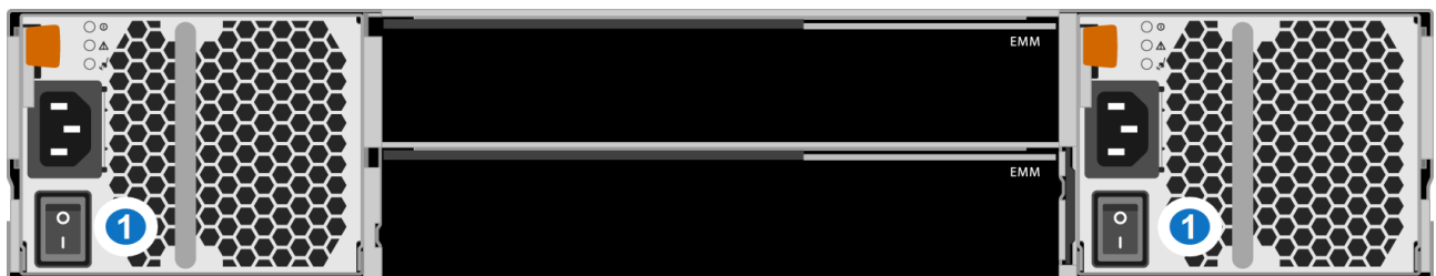
Figure 25: DXi4700 Expansion Module Power Switches
