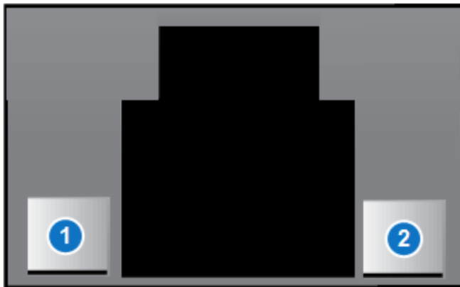
Figure 16: DXi4700 Node - 10 GBase-T Ethernet Port LEDs
