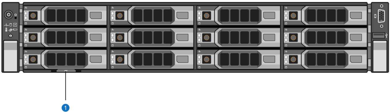
1 - Information Tag Pullout with System Serial Number
