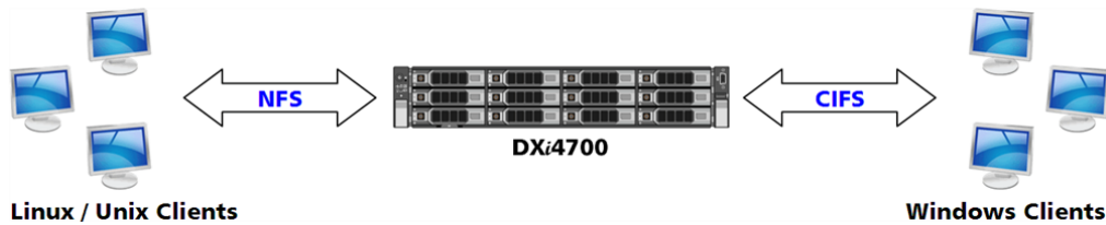
Figure 6: NAS Backup using CIFS and NFS
