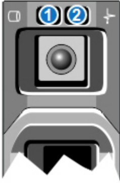
Figure 24: DXi4700 Hard Drive Carrier LEDs
