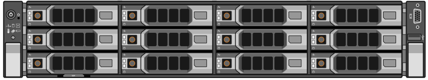
Figure 2 DXi4700 Node Drive Slot Numbering
