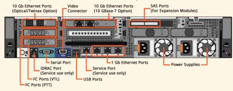
Refer to the *DXi4700 User's Guide*, "DXi4700 Basic Operations" chapter, for additional details about the rear panel components and the optional Ethernet ports.
