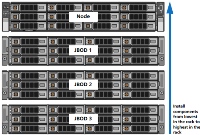
Figure 26: Recommended Component Rack Order (Maximum Configuration)
