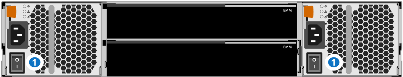
Figure 37: Expansion Module Power Switches
