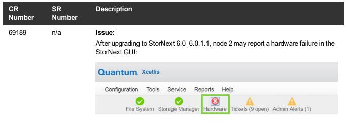
When clicked, this hardware failure displays multiple fan failures on the **System Board** tab of the **Reports > Hardware Status** in the StorNext GUI:
