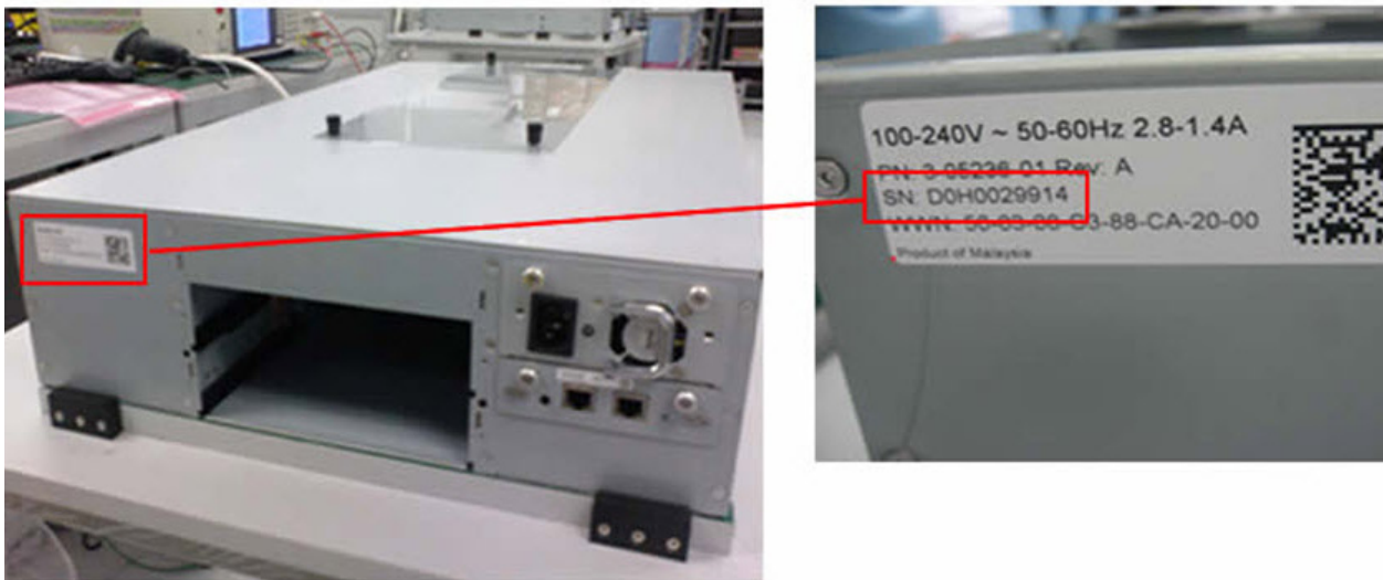
Figure 54 Scalar i40/i80 Serial Number Label and Location
