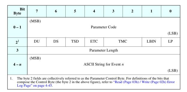
Figure 4-24. Log Parameters Format for Last *n* Error Events LOG SENSE Page
