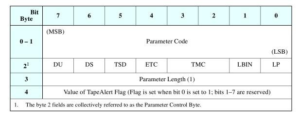
Figure 4-30. TapeAlert LOG SENSE Page — Parameters Format
