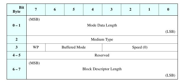
Figure 4-63. MODE SENSE (10) Data Header — Data Format
