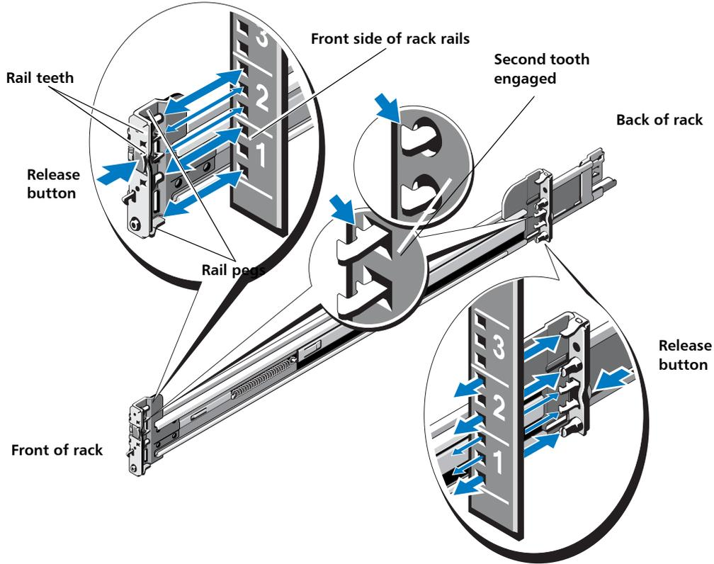
Figure 5 Installing the Rack Mounting Rails (Round Holes)—Right Side Rail view
