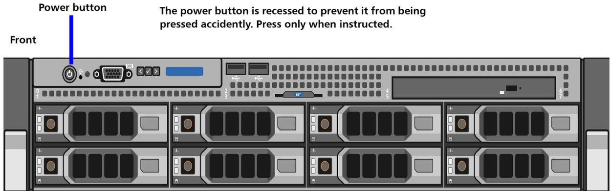
The power button is recessed to prevent it from being pressed accidentally. Press only when instructed.
