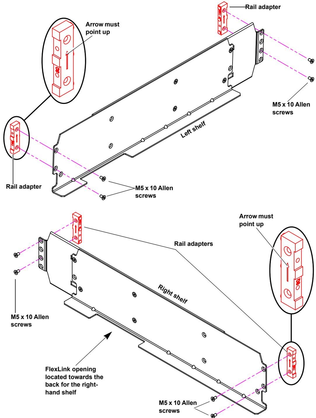
2 Install the left and right rack mount shelves into the rack (the rack mount shelves adjust 27 in. to 36 in.) and secure with the following parts in four locations (see [figure 8](#)):
