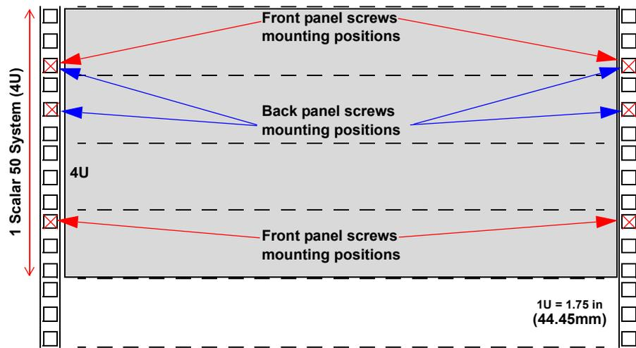
The marks above (X) indicate the location of mounting hardware on the rack rails. Ensure that any necessary mounting hardware is installed on the rack rails prior to installing the chassis.
