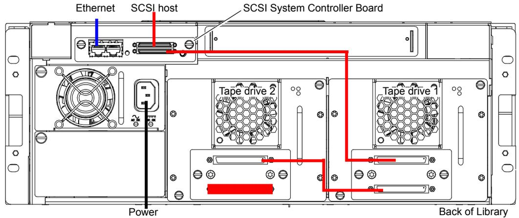
Figure 17 Scalar 50 Cable Configuration (Native Fibre Channel Full Height Drives)
