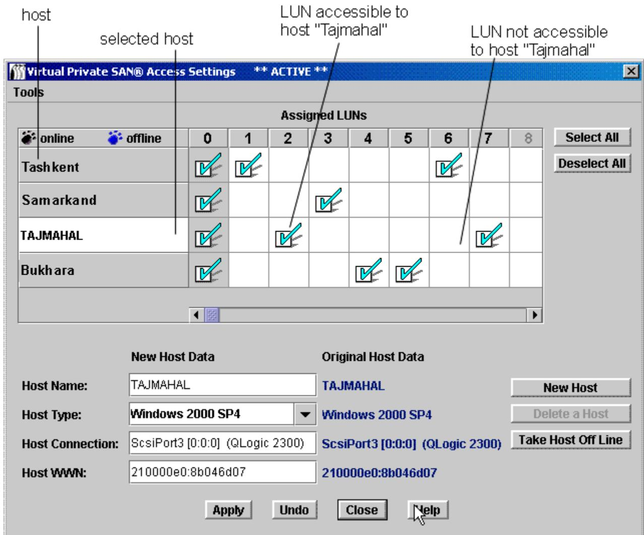
[Figure 22](#) shows labeled components of the **Scalar® Firewall Manager Access Settings** dialog box.
