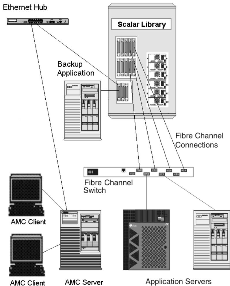
AMC provides several levels of access permissions and the ability to customize views and portals. By keeping track of different client views, you can recall a saved view from any client. The server provides security features by maintaining account names and passwords on behalf of the client application. AMC also provides functionality to support server-less backup, tools for LUN mapping, and easy channel zoning.
