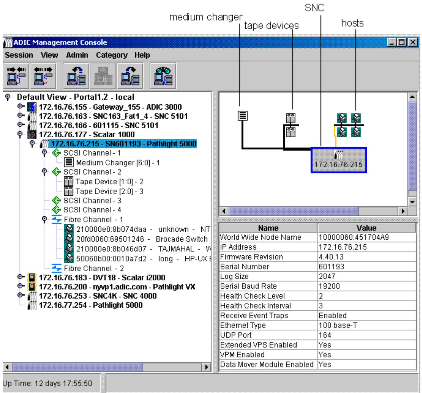
**Figure 3** on page 28 shows a tree panel with several tree elements expanded. Because the SNC 5100 with IP address 172.16.76.215 is selected, it is shown in the tree panel with blue highlighting. This SNC is aggregated into a Scalar 1000. For a list of symbols used in the graphical and tree panels, see **Figure 4**.
