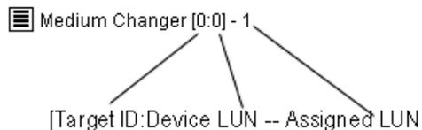
SCSI channels provide target space for IDs 0-15. Device LUNs 0-31 are associated with each ID. The assigned LUN is the LUN the appliance assigns during discovery. The target ID and device LUN are physical concepts.
