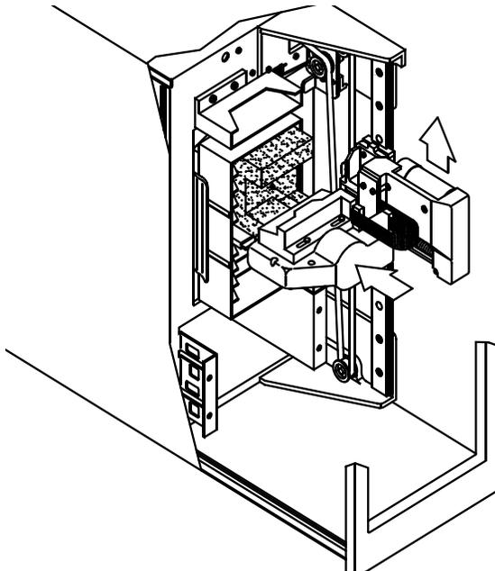
6. Insert the large foam packing piece between the CHM and the door opening, as shown below. Make certain the foam is flush against the upper base of the CHM.
