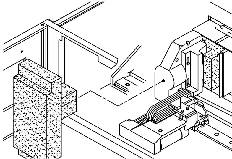
2. To remove the second foam packing piece, you must first move the cartridge handling mechanism (CHM) out and away from the magazine, as described on the next page.
