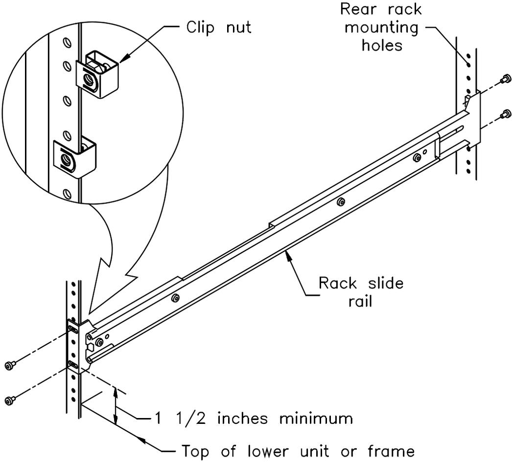
4. Orient the rack-slide rails so that the metal stop is towards the back of the cabinet, as shown in the figure. If the rails are not long enough to reach the back of the cabinet, use a T-15 TORX driver to loosen the nuts on the rails. Extend the rails to the desired length and tighten the nuts.
