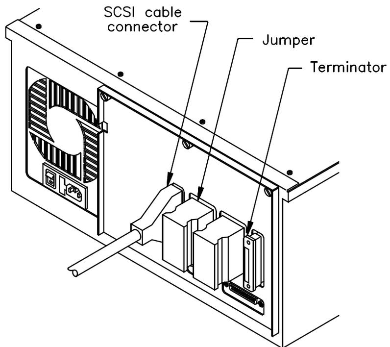
3. For each device that terminates the bus (either the library or one of the tape drives), install a terminator on one of the connectors for that device.
