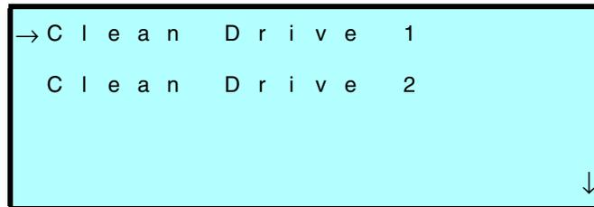
6. Select the tape drive you want to clean. Drive 1 is the tape drive closest to the magazine; Drive 2 is the tape drive farthest from the magazine. When you select a drive, the following activities occur:
