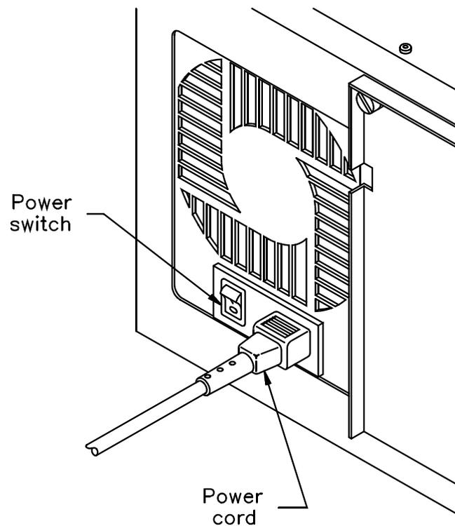
2. Connect the female end of the power cord to the power connector on the back of the library.
