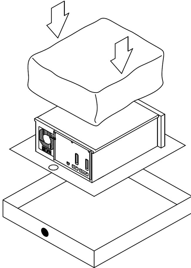
2. Place the cushioned packaging around the library, as shown below. (Use the alignment holes in the packing pieces as a guide.)
