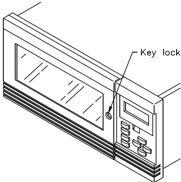
When the CHM finishes the current operation and moves to the park position, the door's interlock mechanism releases.
