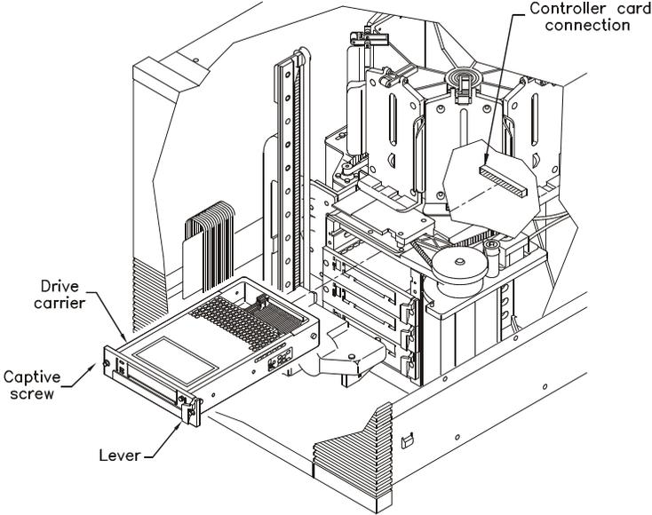
2. When the tape drive is almost completely inside the slot, you will feel some resistance. This is caused by the connection between the tape drive and the library's controller card. **To seat the connection, push firmly against the drive until you can push no further.**
