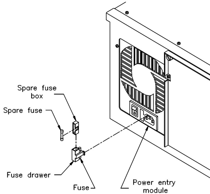
3. Pull the blown fuse out of the fuse slot.
