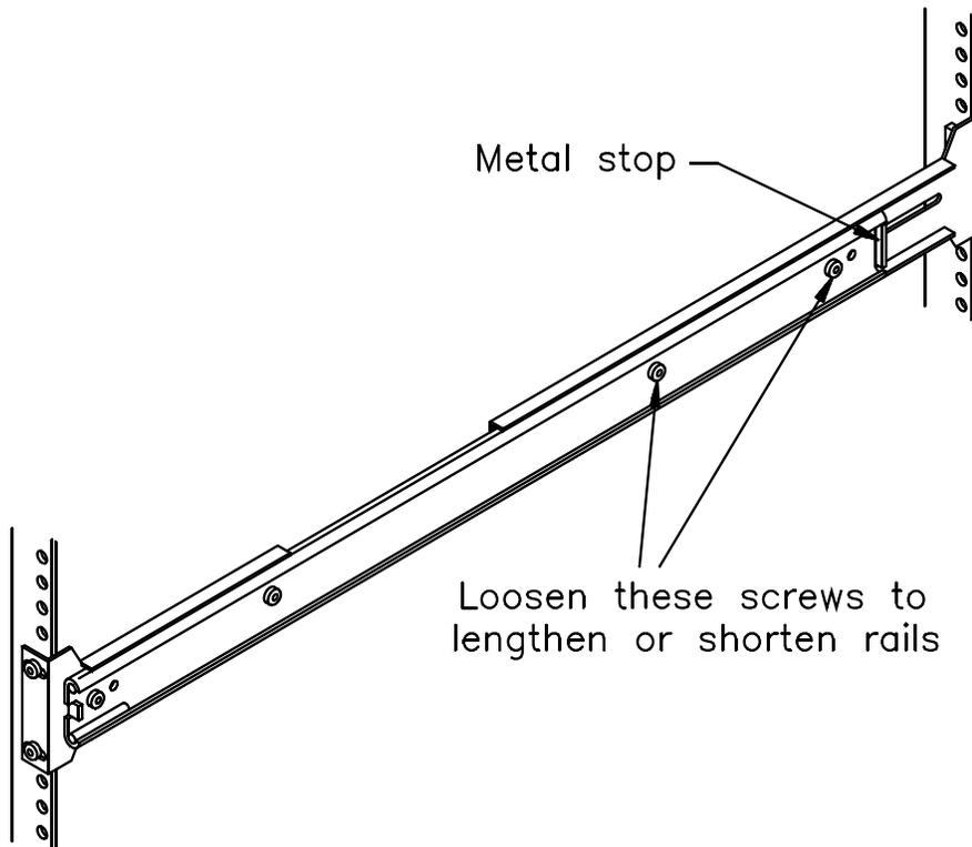
5. Using a T-25 TORX driver and four screws per rail, attach (but do not tighten) the rack slide rails to the mounting holes on the rack, as shown in the figure on page 7.
