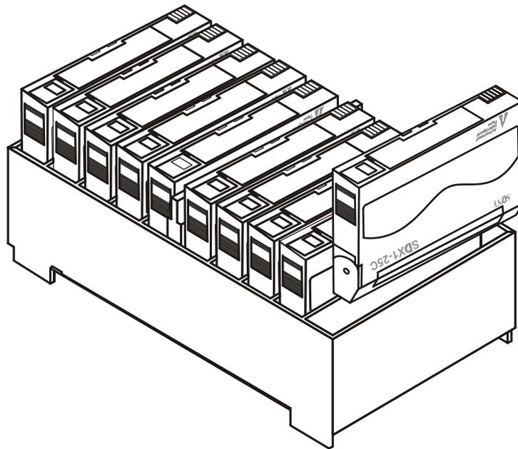
8. The library contains one fixed cartridge slot for a cleaning cartridge or an additional data cartridge. If desired, install a cleaning cartridge in the fixed cartridge slot, as shown on the following page.
