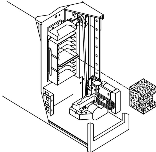
5. Move the CHM so that it is centered in front of the foam packing piece. Push the upper portion of the CHM forward until it is secure between the sides of the foam.
