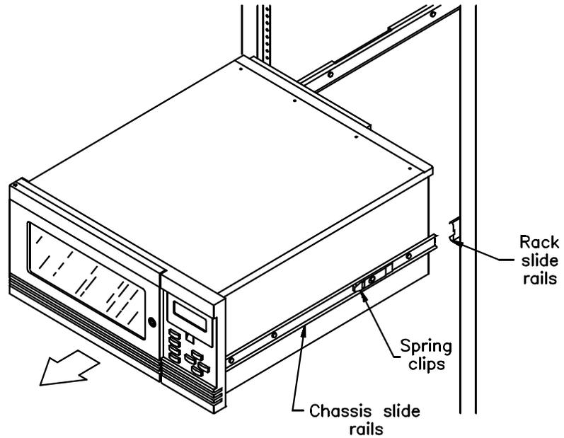
3. If you are shipping the slide rails with the library, use a T-20 TORX driver to remove the four screws that attach each rack slide rail to the front and rear of the cabinet. (See the figure on page 5.)
