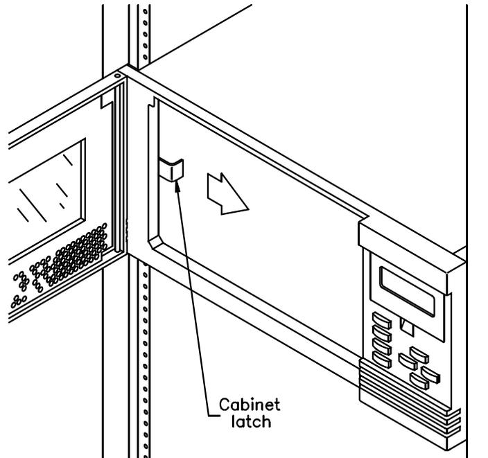
2. Slide the library forward until the rails stop at their spring clips. Using two people, press the spring clips to disengage the rails and lift the library out of the rack.
