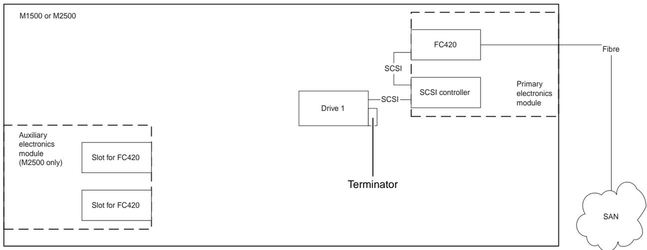
In a one-drive configuration (as shown in [figure 2](#)), a SCSI daisy chain is established from one of the SCSI ports on the FC420 bridge to the SCSI controller and then to drive 1, where the daisy chain is terminated. The SCSI controller is included in the chain to pass SCSI commands to the robot.
