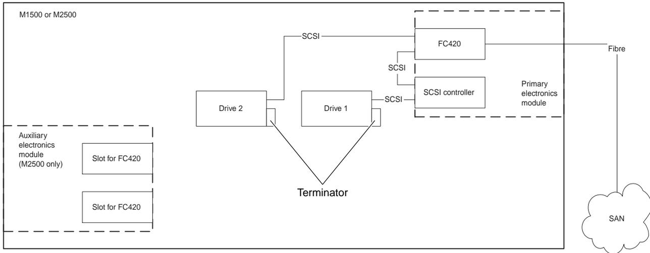
In a two-drive library, the second drive (drive 2) should be connected to the available FC420 port, creating a second SCSI bus. This utilizes the FC420 bridge fully and maximizes the communication bandwidth available to each tape drive.
