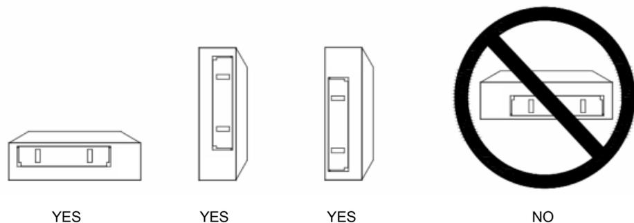
Mount the internal drive in a 5.25-inch, half-height drive bay as follows:
