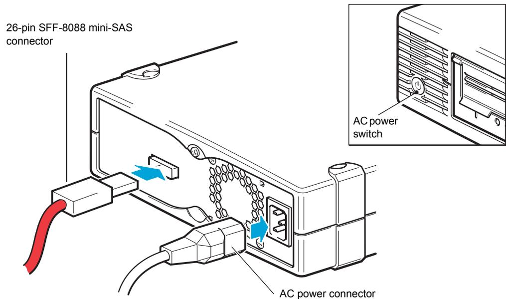
Connect the interface and AC power cables to the tabletop drive as follows:
