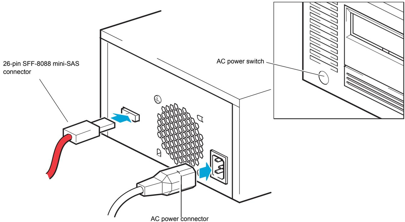
Connect the interface and AC power cables to the tabletop drive as follows:
