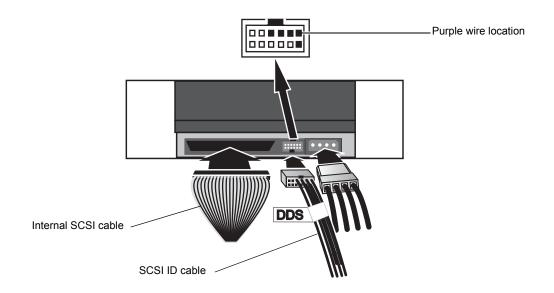
Figure 11 DLT-V4 and DLT VS160 SCSI Connections
