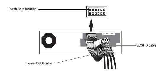
Figure 14 LTO-3 Half-Height Serial-attached SCSI (SAS) Connections
