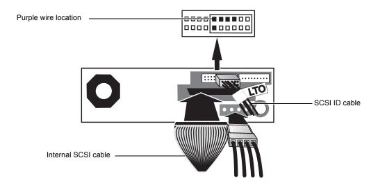
Figure 13 LTO-3 Half-Height Parallel SCSI Connections
