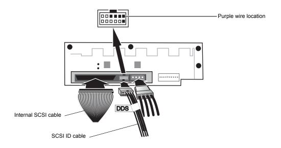
Figure 12 LTO-2 Half-Height SCSI Connections
