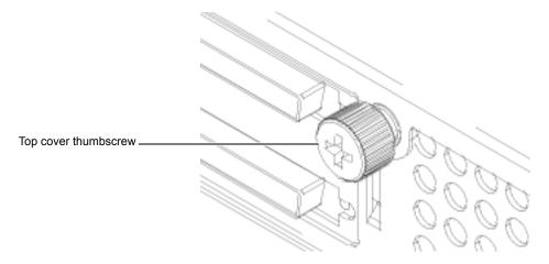
**6** Slide the top cover toward the back of the enclosure about 1/2 inch to disengage it from the front clips and lift the top cover off the enclosure (see <u>figure 6</u>).
