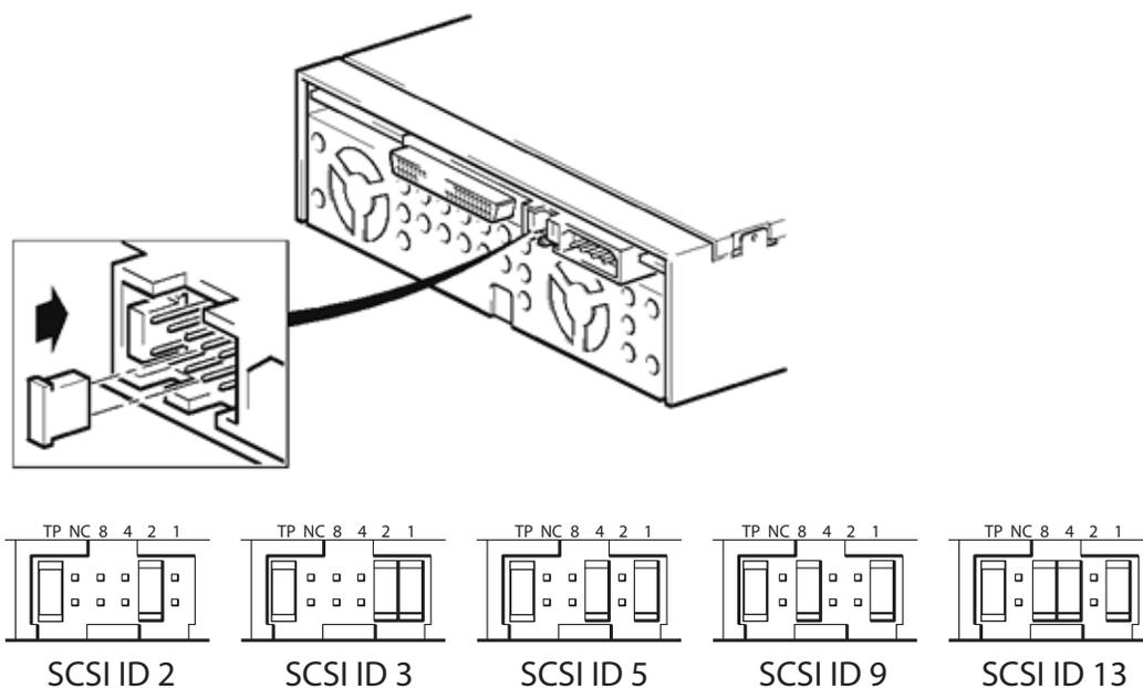
**Note:** Parallel SCSI controllers and host adapters generally use ID 7. In some systems, the boot drive uses ID 0 or ID 1. Avoid configuring the LTO-3 (Model B) Half-Height Tape Drive to these SCSI IDs.
