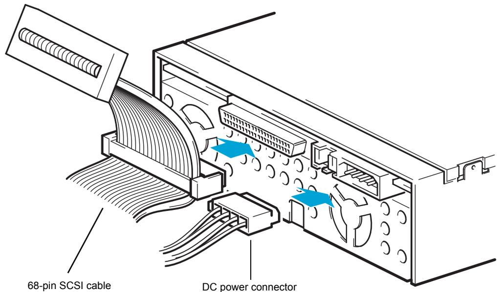
Figure 7 Internal SAS Drive Interface and DC Power Connectors
