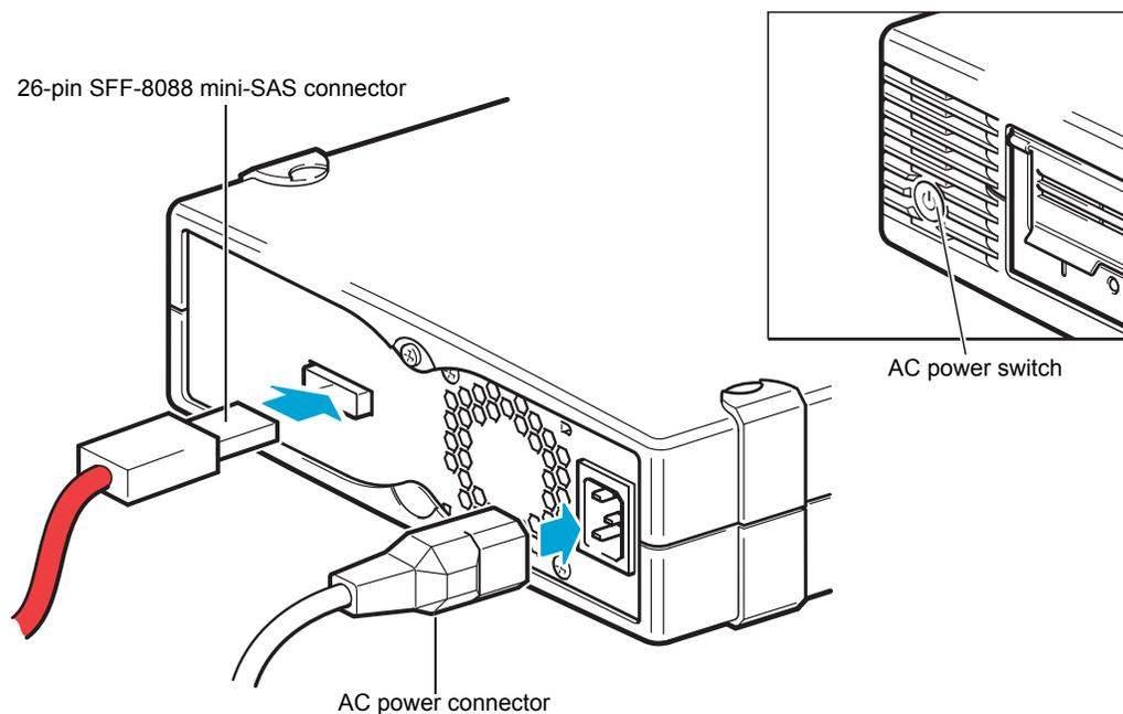
Connect the interface and AC power cables to the tabletop drive as follows:
