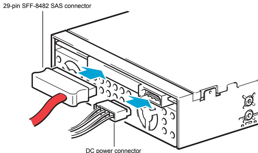
Connect the interface and DC power cables to the internal drive as follows:
