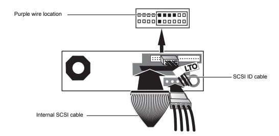
Figure 13 LTO-3 Half-Height Parallel SCSI Connections
