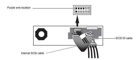
Figure 14 LTO-3 Half-Height Serial-attached SCSI (SAS) Connections
