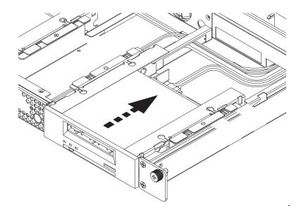
Figure 18 Reinstalling the Mounting Bracket Screws
