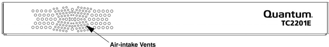
The air intake vents shown in [figure 1](#) provide cooling for the unit during operation and should always remain unobstructed. The exhaust vent for air is located on the back panel.
