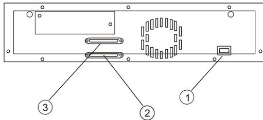
**4** To power up the autoloader, use the eraser end of a pencil or something similar to press the left side of the power switch.
