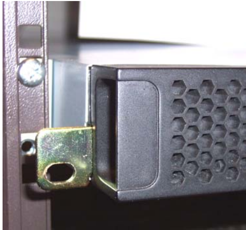
Figure 3.5 Slide the FastStor 1 in from the front
