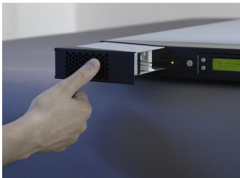
Figure 4.20 Push magazine until it clicks into place
