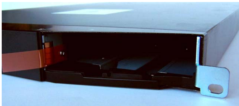
Figure 6.1 Transport lock marked with red plastic tab
