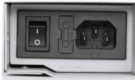
Figure 3.8 Power switch, fuse holder and power cord connection
