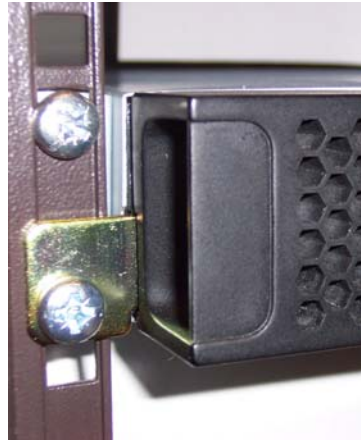
Figure 3.6 Fasten the front of the FastStor 1 to the rack
