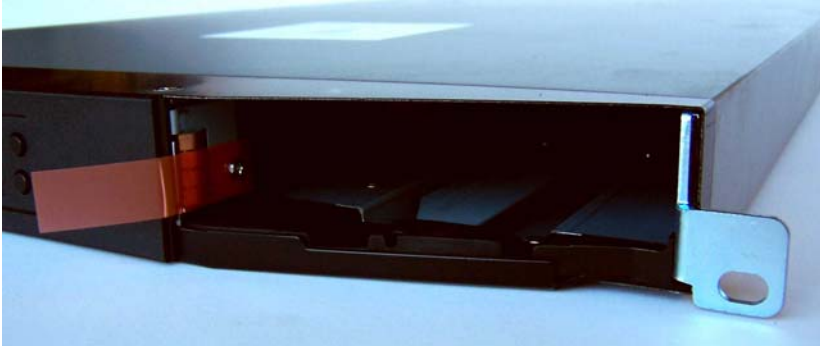
Figure 3.9 Magazine lock marked with red plastic tab
