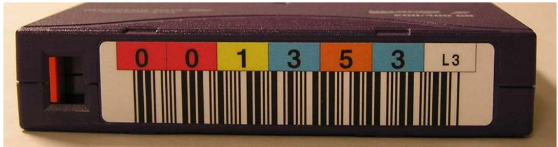
Figure 3.11 Positioning of barcode label for LTO cartridges.
