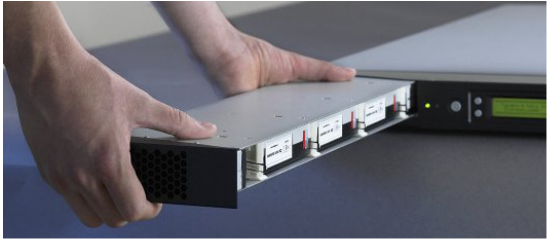
Figure 4.16 Removing the magazine from the loader
