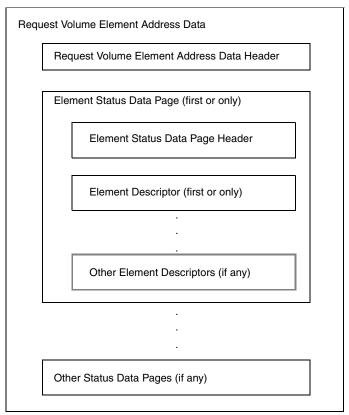
A single **Volume Element Address Header** is returned along with 1 or more element status pages. The **Volume Element Address** indicates:
