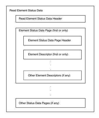
A single **Read Element Status Data Header** is returned along with one or more element status pages. The **Read Element Status Data Header** indicates the address of the first element reported, number of elements reported, and the report size for all requested data.
