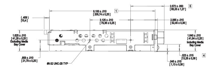
Figure 2-2. Mounting Holes and Dimensions (Side View)
