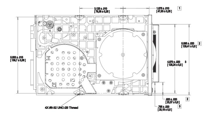
Figure 2-1. Mounting Holes and Dimensions (Bottom View)
