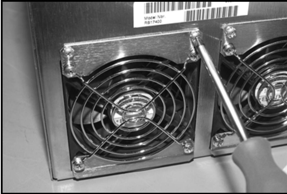
*Figure 3.4 Fan Removal*
