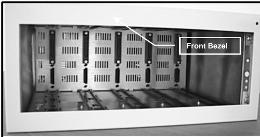
*Figure 1-1: T5 Enclosure, Front View*
