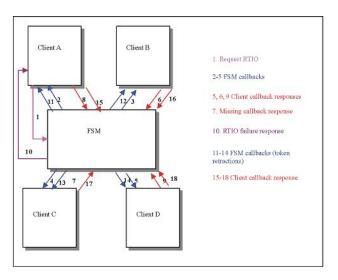
In Figure 77, Client A requests some amount of **RTIO** as in Figure 76. However, assume that Client C did not respond to the initial callback in time (step 7). The FSM will return a failure to Client A for the initial **RTIO** request, then send out callbacks to all clients indicating the stripe group is no longer real-time (steps 11-14). In the example, Client C responds to the second callback, so the FSM will not send out any more callbacks. The stripe group is back in non-real-time mode.
