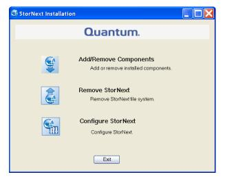
If you previously installed StorNext and would like to add or remove components, display the **StorNext Installation** window by doubleclicking the file named **SnfsSetup64.exe** (64-bit systems). Note that the screen is slightly different from Figure 46 above: instead of Add/ **Remove Components**, the button you need to click is called **Upgrade/Reinstall StorNext** (see Figure 47).
