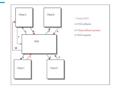
In the above diagram, a process on client A requests some amount of **RTIO** in Step 1. Since this is the first request, the FSM issues callbacks to all connected clients (Steps 2-5) informing them that the stripe group is now in real-time mode. The clients respond to the FSM in Steps 6-9. After all the clients have responded, the FSM responds to the original requesting client in Step 10.
