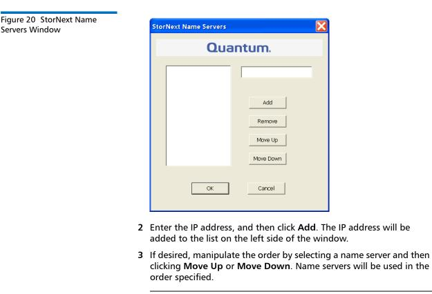
**Note:** The Name Servers configuration (including the ordering) must be identical on all computers running StorNext.
