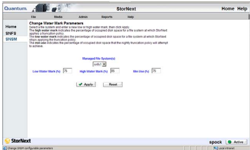
Figure 148 Change Watermark Parameters Screen
