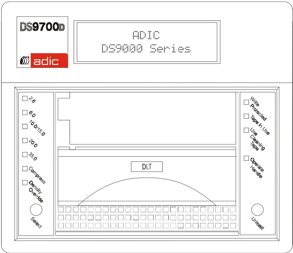
Figure 2. DS9700D Front Panel
