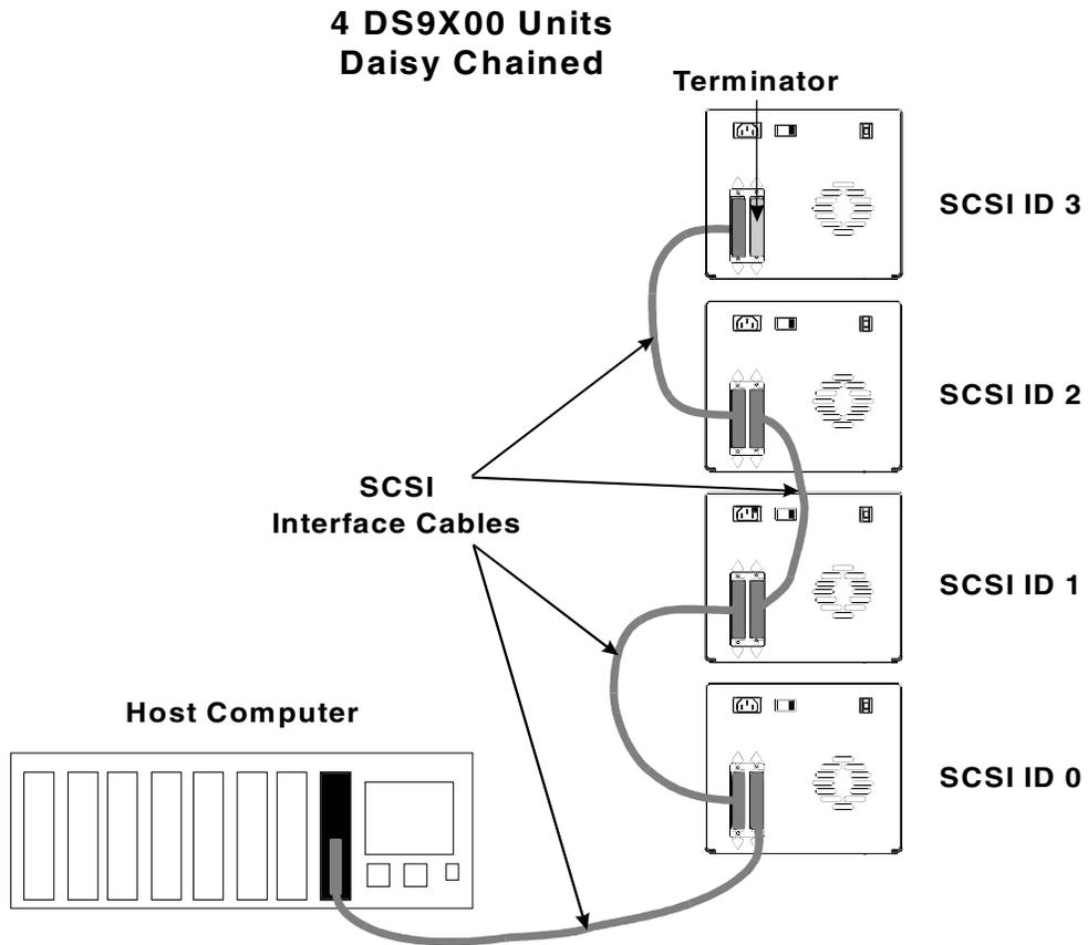
Figure 6. Cable Diagram for 4 DS9000 Series Units
