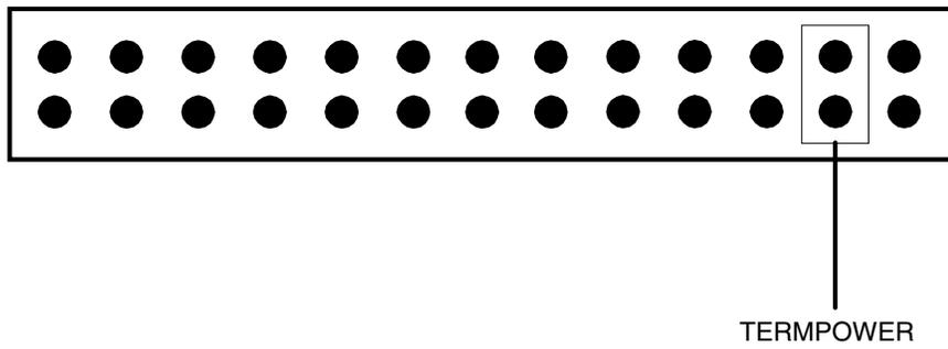
Figure 16. Term Power Pins on TRM PWR Connector
