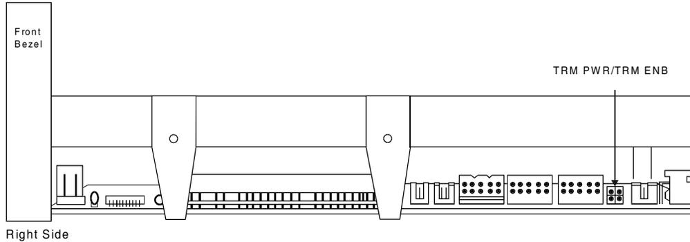
*Figure 13. DLT4000 Tape Drive Connectors (right side)*
