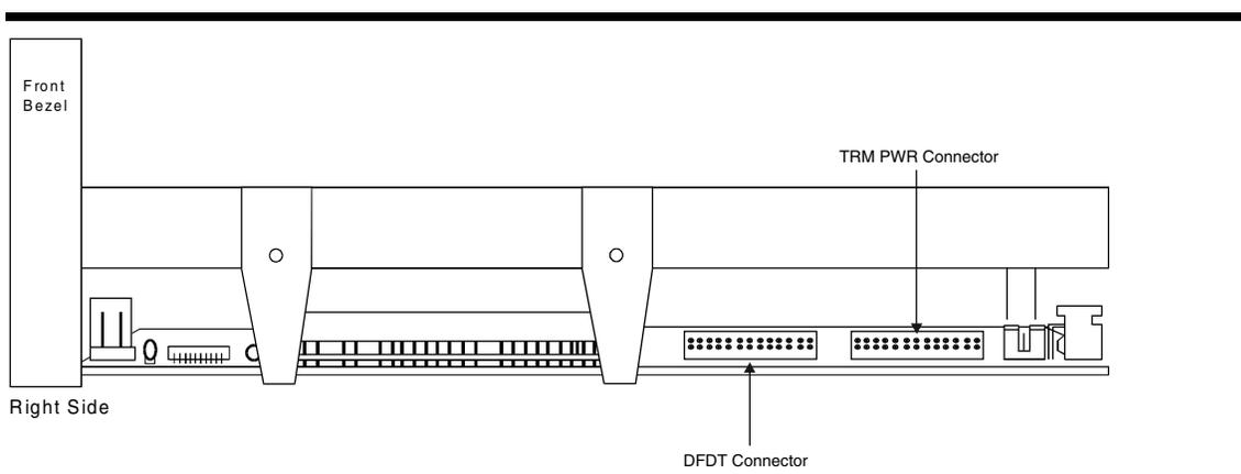
Figure 15. DLT7000/DLT8000 Tape Drive Connectors (right side)
