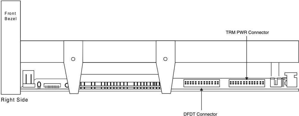
Figure 11. DLT7000/DLT8000 Tape Drive Connectors (right side)
