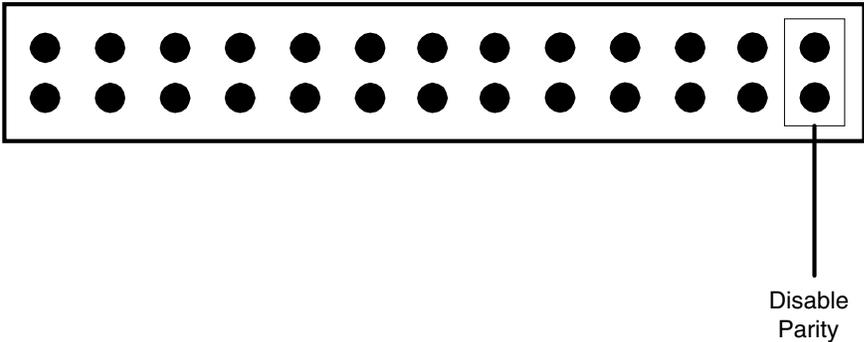
Figure 12. Disable Parity Pins on DFDT Connector
