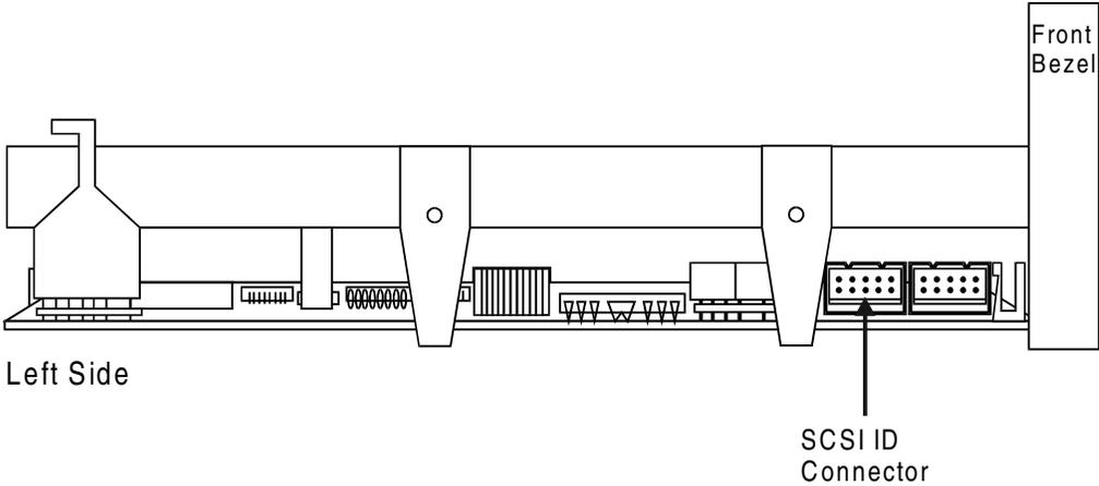
Figure 9. DLT4000 Tape Drive Connectors (left side)
