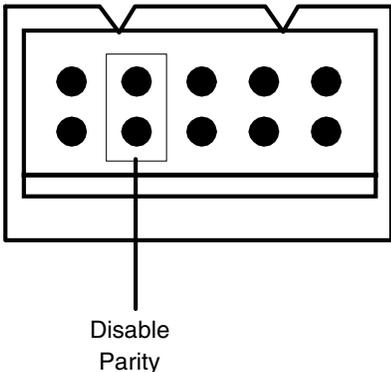
Figure 10. Disable Parity Pins on SCSI ID Connector
