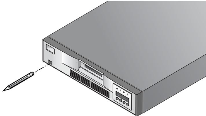
**Note:** The power switch lets you turn the power on and off for the autoloader and the enclosed tape drive. The power switch is recessed into the front panel to prevent the autoloader from being accidentally turned off during operation.
