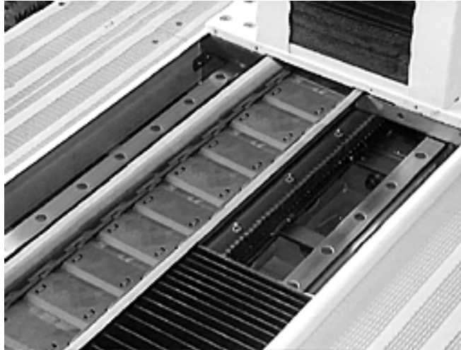
Figure 2-3 Track Section Shown with Cable Chain
